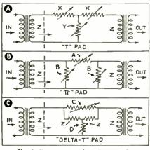
Fig. 2. Three constant-impedance pads.
